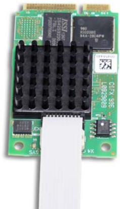
Figure 50: Connecting the CANopen Assembly Interface (AIFX-CO) to the basic Card CIFX 90E (Example)
