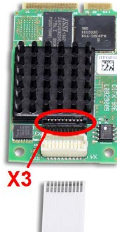
Figure 50: Connecting the CANopen Assembly Interface (AIFX-CO) to the basic Card CIFX 90E (Example)
