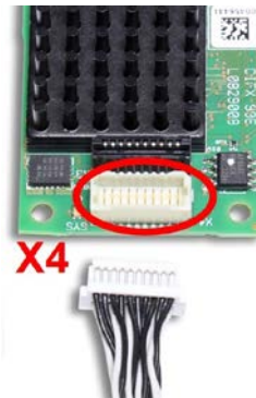
Figure 49: Connecting the Ethernet Assembly Interface (AIFX-RE) to the basic Card CIFX 90E (Example)
