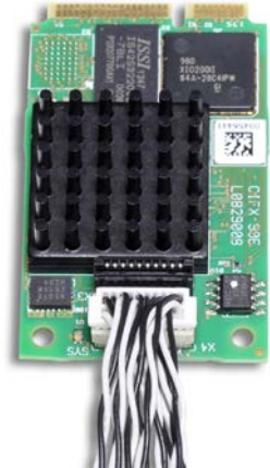
Figure 49: Connecting the Ethernet Assembly Interface (AIFX-RE) to the basic Card CIFX 90E (Example)
